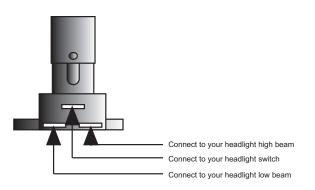
Connect the Dimmer Switch wires as shown above.
